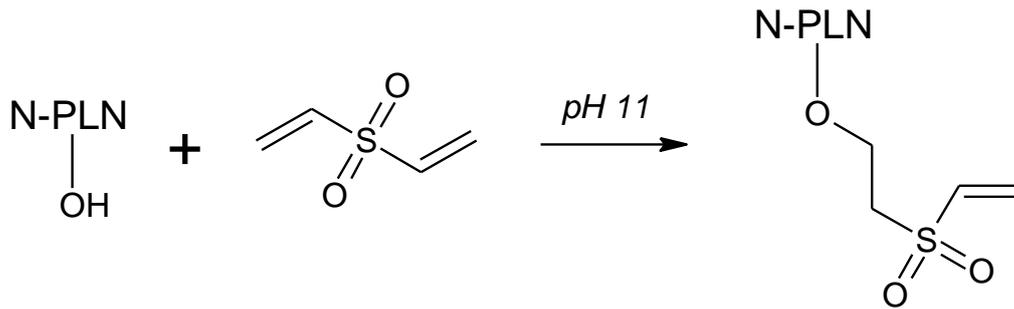
Figure 2: Base-catalysed Michael Addition reaction between hydroxyl groups of Pullulan and Divinylsulfone.
